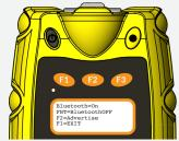
Press '6' on the keypad to select pairing settings. Press ENTER on the keypad to turn pairing on. Ensure that the top line now reads 'Bluetooth=ON". Press F1 to exit the menu.
