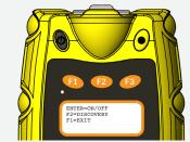
Once in the tool setting screen, the following functions are accessible; press ENTER to toggle pairing ON/OFF, press F2 to activate discovery mode, press F1 to exit the menu.
