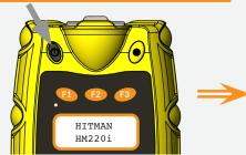
Press the ON button once to switch on. To power OFF: press and hold Power button until the red led comes on or screen turns off. HM200i will power off automatically after 30s.
